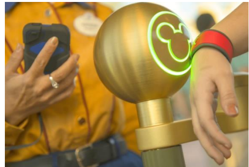
Disney World RFID/NFC MagicBand being read for access authorization
